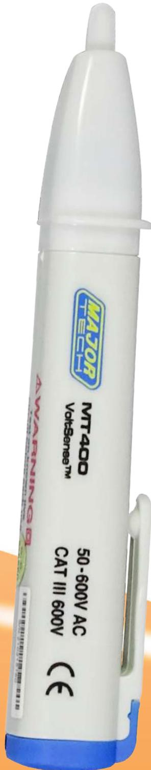
Use MT400 to quickly check for the presence of live wires before performing any electrical testing. Suitable for outlets or against wire insulation testing, this AC Voltage Detector for non-contact detection of AC Voltage from 50 to 600V (50/60Hz). The Red LED in the tip indicates the presence of voltage.
