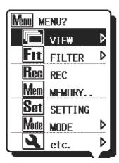
Move the cursor with the UP/DOWN Keysr Shuttle Switch, and confirm the selection with the ENTER Key. Pressing the ESC Key while the Menu is being displayed closes the Menu Window. Items displayed with "p" mark are accompanied with submenus. Press the ENTER Key to access to the submenus.
