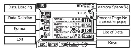
Functions to recall  $\Leftrightarrow$  displays the saved data), delete  $\Rightarrow$  deletes the saved data) and format the data  $\Rightarrow$  formats the internal memory ) are available. Details of each parameter are as follows.
