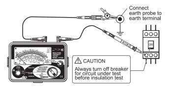
① Check the circuit under test is not energized as follows. Connect the test probe to the circuit under test and read a voltage value. If the circuit is live, the meter indicates the voltage, the live circuit lamp is lit, and warning buzzer sounds.
